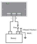
Figure 3-3 Battery connecting
