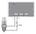
Figure 3-4 Load Wiring
