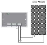
Figure 3-5 Solar wiring
