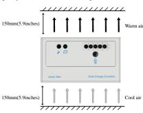
Figure 3-1 Mounting and cooling
