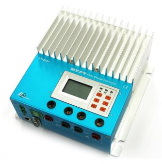
eTracer is an advanced Maximum Point Tracking (MPPT) controller for off-grid photovoltaic (PV) systems up to 3KW. The controller features a smart tracking algorithm that maximizes the energy harvest from the PV by rapidly finding the solar array peak power point in all the weather condition. The controller provides higher efficiency up to 98% with lower power loss.
